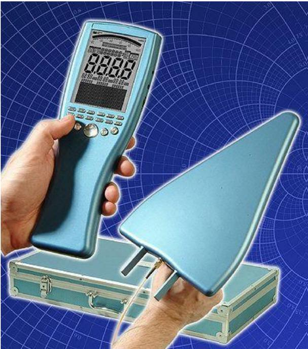
**Figure 2 - Spectran HF6060 with HyperLOG 7060 Antenna Used for Narrowband Measurement (Source: [www.spectran.com](http://www.spectran.com))**
