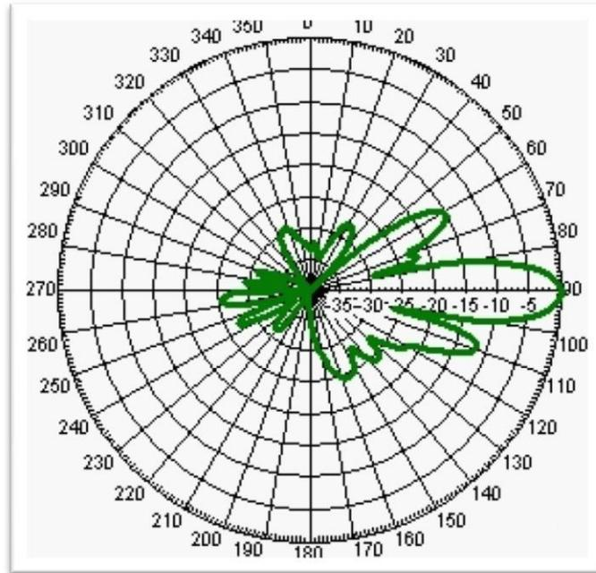
**Figure 25 - Vertical Radiation Pattern for a Typical Base Station Antenna (Source: [www.commscope.com](http://www.commscope.com))**
