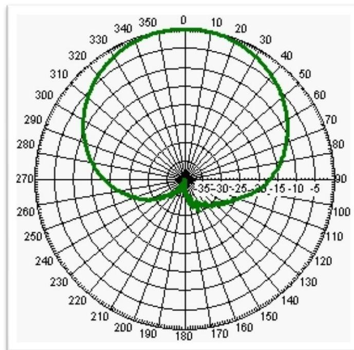
**Figure 26 - Horizontal Radiation Pattern for a Typical Base Station Antenna (Source: [www.commscope.com](http://www.commscope.com))**
