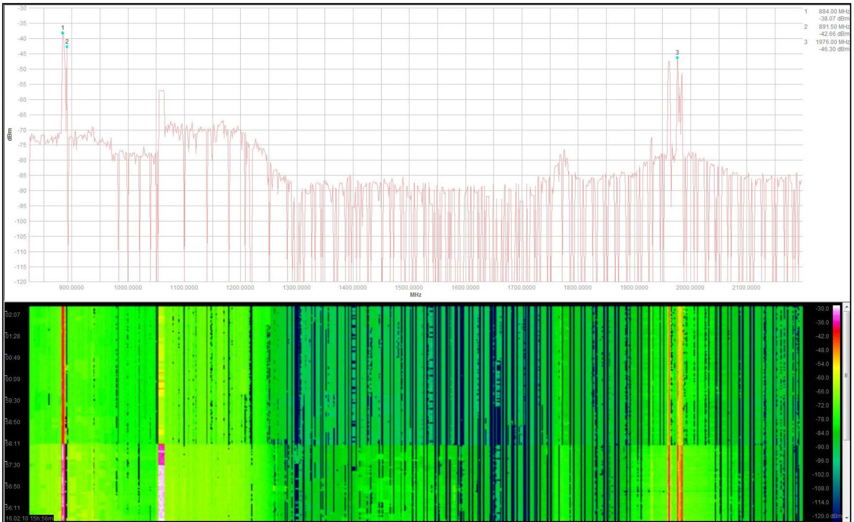
**Figure 4 - Narrowband Measurement Example (10-minute sweep 800MHz – 2200MHz)**
