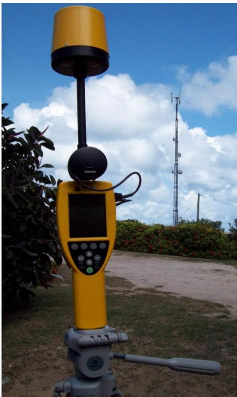
**Figure 1 - NBM-550 with ED5091 Probe used for Broadband Measurement**
